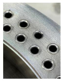
"As you execute these welds, you have to make sure to balance the heat load on the part," said Schwartz. "That means you can't weld more than two tubes around the same location at once; otherwise, you have a very hot area, and the part will deform."
