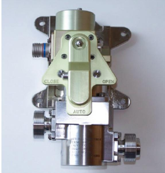
Part number 12085-5 is used on the International Space Station in the Hydrogen Vent Assembly and Major Constituent Analyzer in the Environmental Control and Life Support System. The valve is totally pressure balanced using edge welded Inconel bellows.
