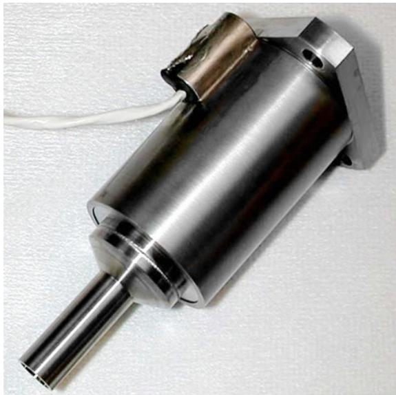
Part number 15027 is a dual seat propellant control valve qualified for thrusts from 50 to 100 LBf. Derivative designs will fly on VEGA, Mars Science Laboratory and other U.S. Government Programs. These designs use ValveTech's patented Center Guide Technology for high cycle life and reliability. They are all welded stainless steel construction and use an AF-E-411 puck in an annular type seat for seat sealing.
