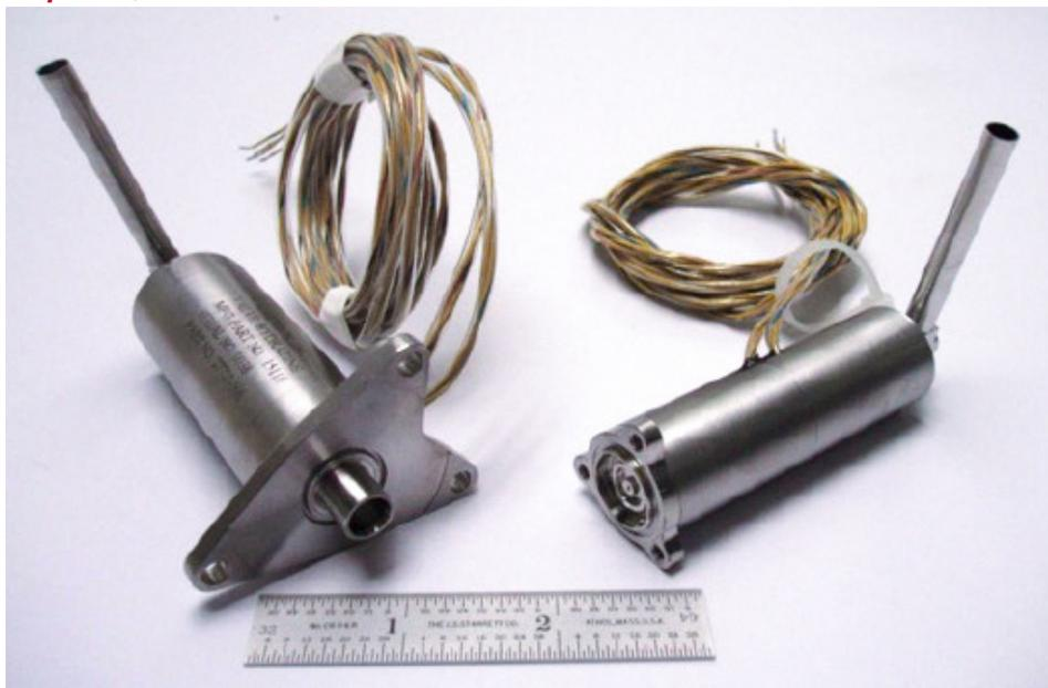
*ValveTech has qualified and flown a number of propellant control valves for small, monopropellant rocket engines in the 0.1 to 5.0 Lbf. range. The valve design uses an AF-E-411 elastomeric puck for exceptional sealing capability.*
