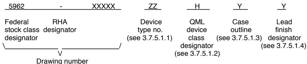
3.7.5.1.1 Device type. The device type shall identify the circuit function as indicated in the SMD.
