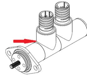
Electromech's next challenge was a part design that, as initially planned, would require 7 different welds, including 2 saddle welds.
