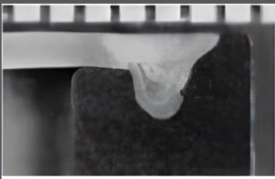
Figure 1e, top view of nickel-and gold-plated Kovar butt weld.
