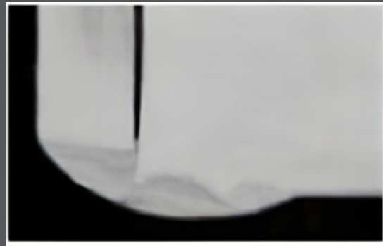
Figure 1b, cross-section of a butt weld in the stainless-steel relay in figure 1a, weld penetration is 0.008"
