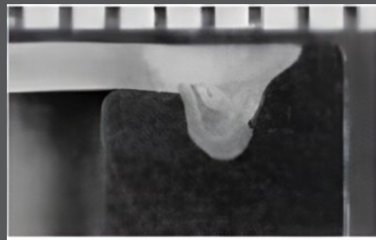
Figure 1f, weld cross-section of drop-in cover shown in figure 1e. Weld penetration is 0.025".
