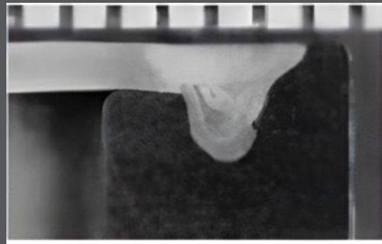
Figure 1d, weld cross-section of drop-in cover shown in figure 1c. The cover is 0.02" thick 4047 aluminum and the housing is 6061 aluminum. Weld penetration is 0.47".
